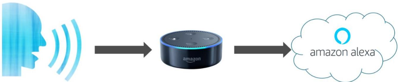
When the microphone button is pressed, it turns red, and the microphone is off. The Echo device stops listening completely and will not respond to the wake word or respond to the action button until you reactivate it by pushing the microphone button again. The microphone cannot be turned back on remotely or by software.
