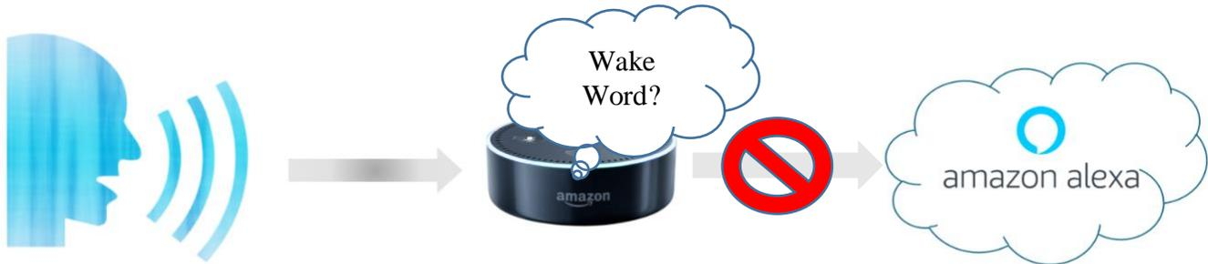
When the Echo device detects the wake word, it streams audio to the cloud, including a fraction of a second of audio before the wake word. The light ring around the top of the device turns blue, to indicate that the device is streaming audio to the cloud. The audio streaming stops and the blue light turns off when the Echo device detects a pause or when Alexa has enough information to process a command.
