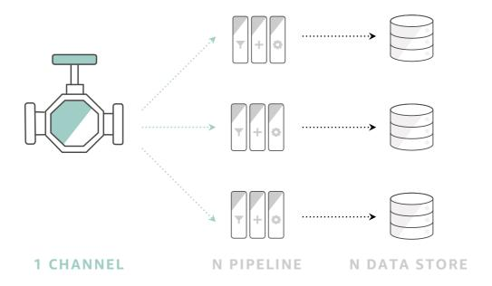
This type of configuration replicates the messages at the channel output. Each pipeline is presented with the same raw message as received by the channel. Thus, a channel over here acts as a broadcaster device.
