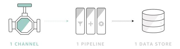
For the simplest way to leverage channels and pipelines, it's best for all messages to follow the same structure, JSON. This helps us keep our pipeline operations simple. For multi-schema messages, this requires a more complex pipeline architecture or include a lambda function to ensure data is processed correctly.
