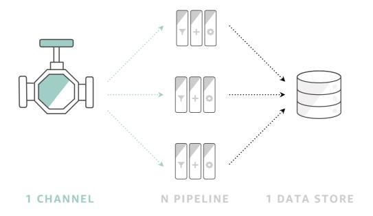
Like in previous data flow types, the messages are replicated at a channel level. Each pipeline is presented with the same raw message as received by the channel.
