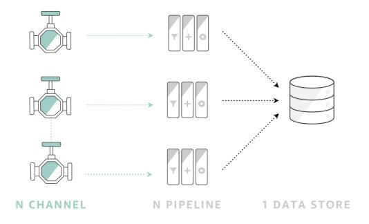
For the type of use case, where we want to perform analysis on different attributes originating from different sources and in different schemas, we can design dedicated pipelines for transformation of multischema messages. This kind of design allows us to store relevant data in one data store.
