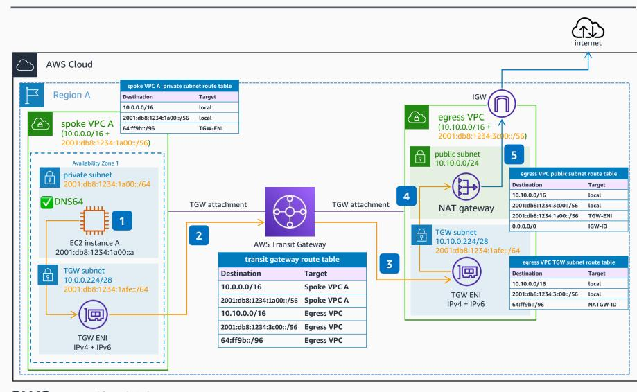
You need to enable DNS64 in all the subnets where you want your IPv6-only workloads to talk with IPv4-only destinations. That way, the **Amazon Route 53 Resolver** looks up the DNS record for the service queried. If there is no IPv6 address associated with the destination, it synthesizes one by prepending the well known 64:ff9b::/96 prefix, to the IPv4 address in the record.
