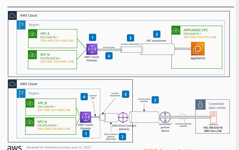
For **Transit Gateway** connect configuration, configure the transit gateway CIDR block. You can specify a size /24 CIDR block or larger for IPv4, or a size /64 CIDR block or larger for IPv6.
