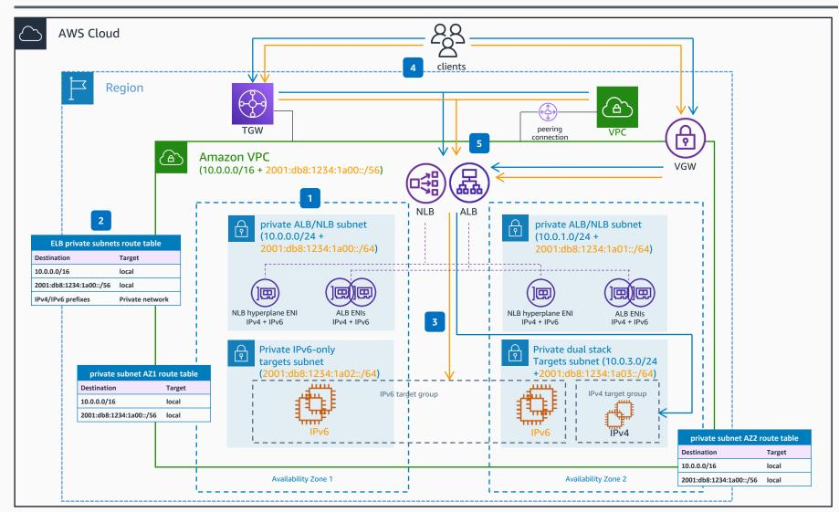
Configure your VPC NLB or Application Load Balancer (ALB) subnets as dual stack, to accommodate for the internal Elastic Load Balancing (ELB) instances..
