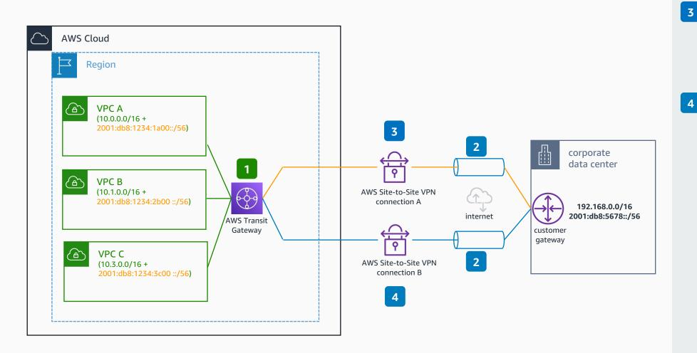
To configure dual stack support for VPN, create two transit gateway VPN attachments, one for each IP stack.
