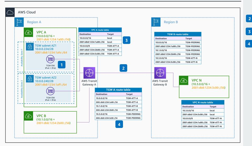
When you attach a VPC to an **AWS Transit Gateway**, you must specify one subnet from each Availability Zone to be used by the **Transit Gateway** to route traffic. For dual stack support, the **Transit Gateway** attachment subnets must have IPv6 CIDR blocks associated, and the attachment must be enable for IPv6 routing.
