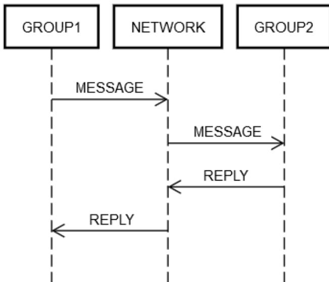
One way or another, some machine within GROUP1 has to put a message on the network, NETWORK, addressed (logically) to GROUP2. Some machine within GROUP2 has to process the request, and so forth. The fact that GROUP1 and GROUP2 are comprised of groups of machines doesn't change the fundamentals. GROUP1, GROUP2, and NETWORK can still fail independently of each other.
