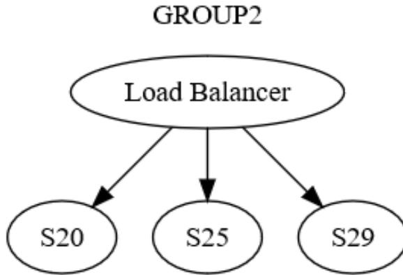
At first, a message to GROUP2 is sent, via the load balancer, to one machine (possibly S20) within the group. The designers of the system know that S20 might fail during the UPDATE STATE phase. As a result, S20 may need to pass the message to at least one other machine, either one of its peers or a machine in a different group. How does S20 actually do this? By sending a request/reply message to, say, S25, as shown in the following diagram.
