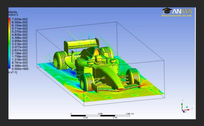
External flow over a Formula-1 Race Car (140M cell mesh)
