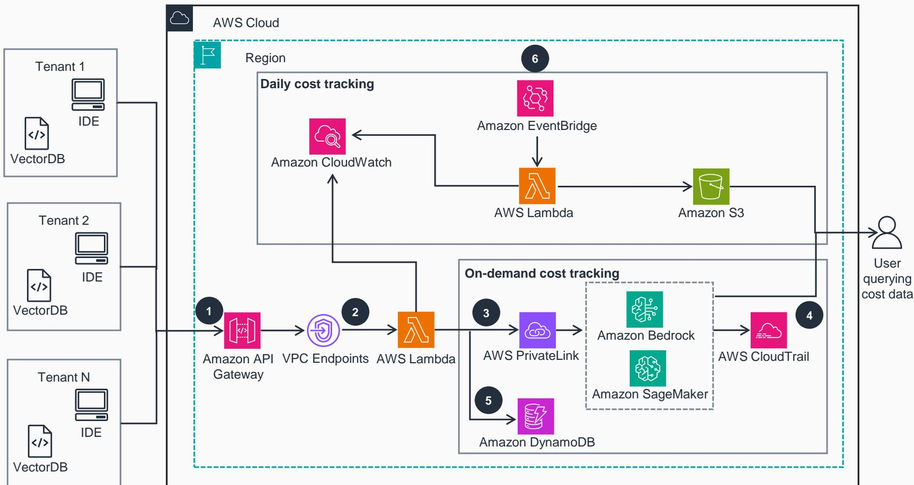
**1** The Software-as-a-Service (SaaS) [AWS Cloud Development Kit \(CDK\)](#) template deploys all required resources to the AWS account. After deployment, a tenant's application sends a POST request to [Amazon API Gateway](#), invoking a specific model by passing the `model_id` as a request parameter and the appropriate model payload in the request body. The tenant can be an individual user, a specific project, a team, or even an entire department within a company.
