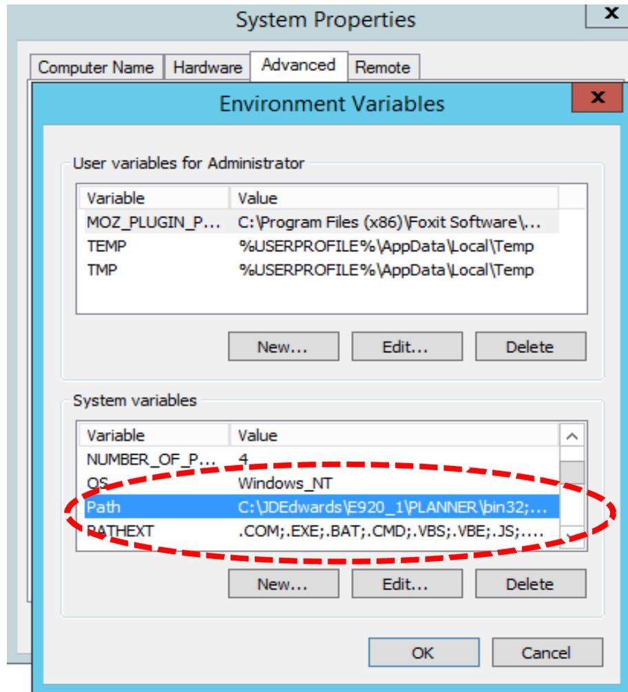
Figure 21: Path system variable
