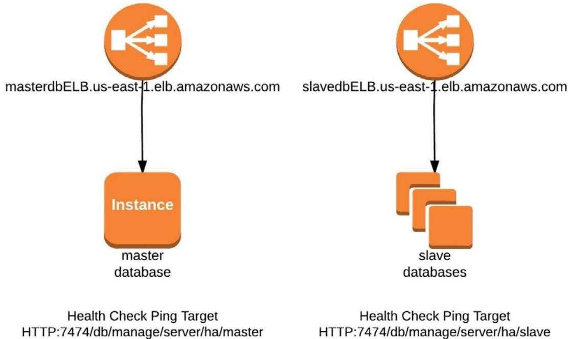
**Figure 3: Neo4j cluster REST endpoints for the master node and the slave nodes**
