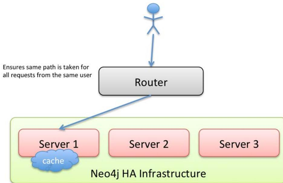
**Figure 4: Solution architecture for consistent routing**
