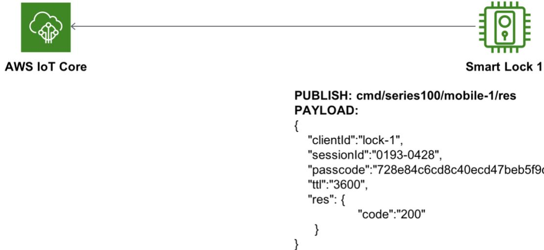
Figure 10: Smart lock response published to AWS IoT Core
