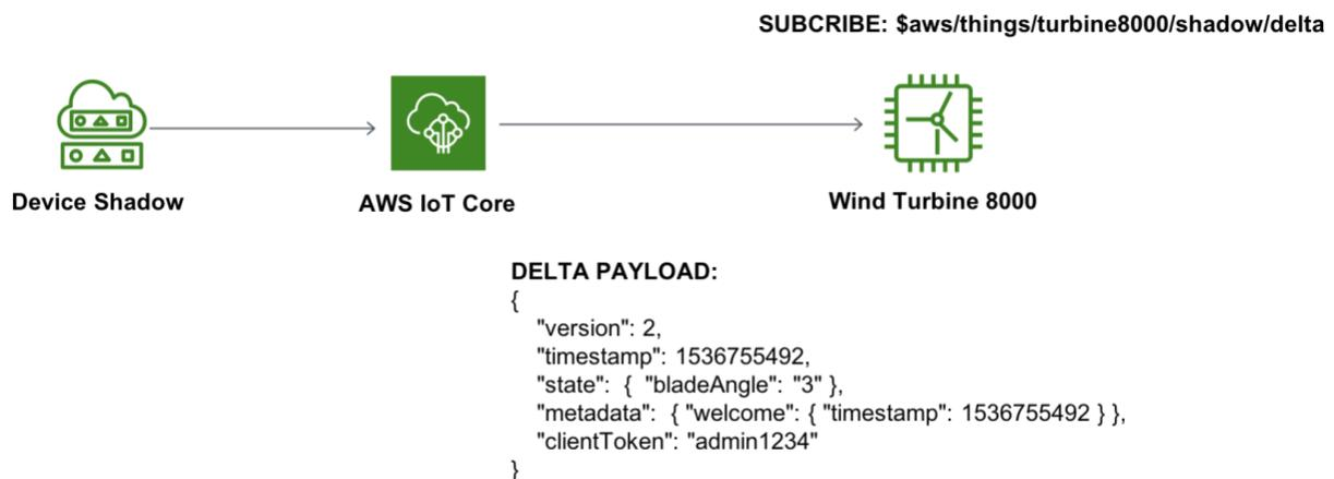
Figure 6: Command processing on wind turbine
