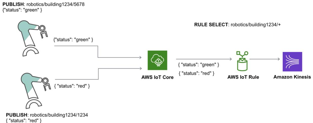
Figure 4: Many-to-one communication in fan-in pattern
