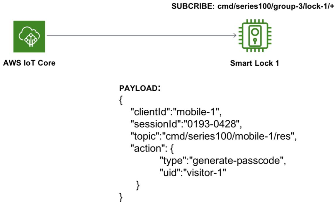
*Figure 9: Command sent from the AWS IoT Device Gateway to the smart lock*
