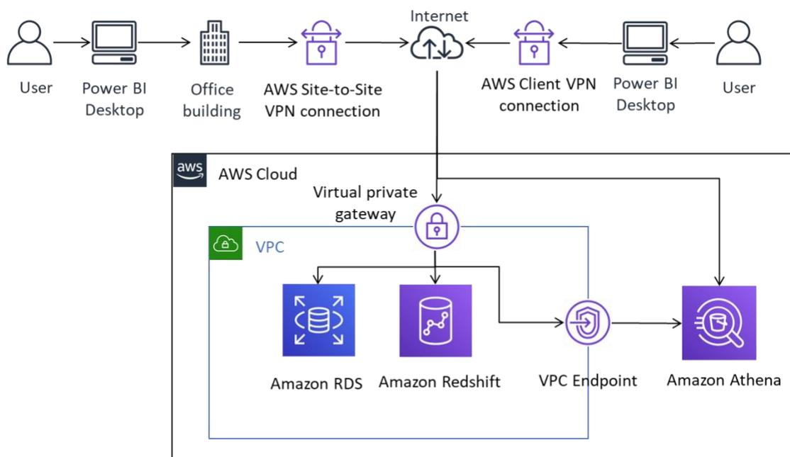
Figure 2 – Connecting Power BI Desktop to AWS data sources over Site-to-Site VPN and Client VPN
